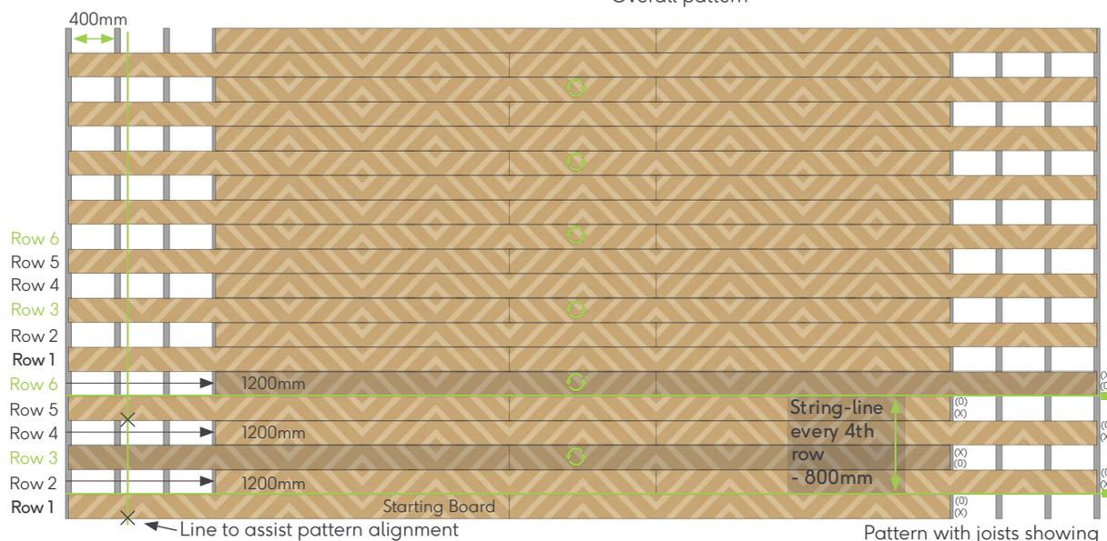
Pattern with joists showing
