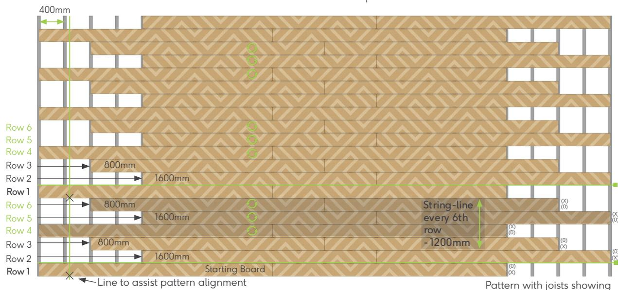
Pattern with joists showing
