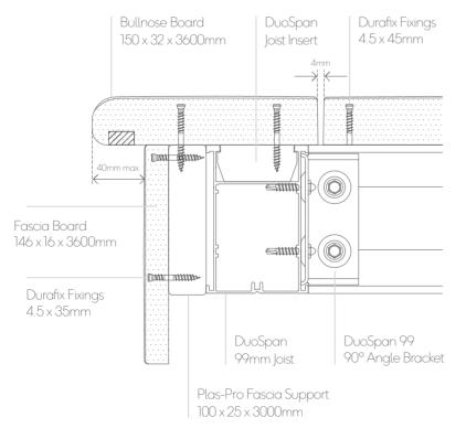
$\ref{M}$  Max. recess area for LED strip lighting is 17 x 9mm, up to 11mm from the fascia.
