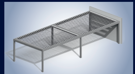
Example: Wall coupling on the long side
